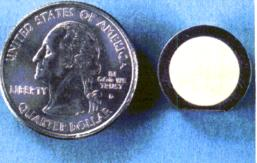
mm in diameter and 6.25 mm in miniature D-shaped antenna can be used in handheld terminals for WLANs and
