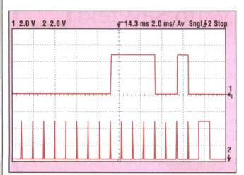
3. This oscillograph shows the data and clock of the R counter.
