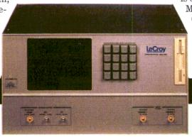
plifiers. A source synthesizer The MCA1060 communications analyzer has a generates signals to stimulate 6.40-in. (16.26-cm) color screen and a built-in devices under test (DUTs), floppy-disk drive.
